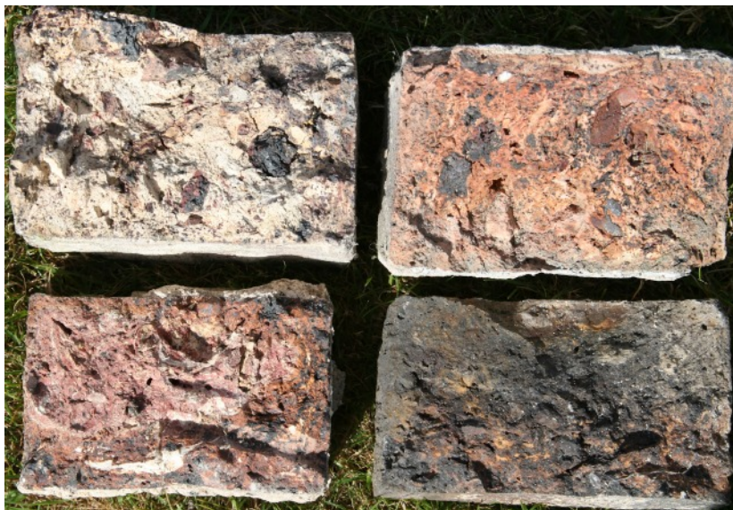
Four examples of inclusions in the interior of Broseley bricks
