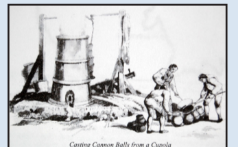
Cupolas are still used today and are typically 'all' heights up to about 20m. The 1803 version shown here is casting cannon balls. Image courtesy of the IGMT
