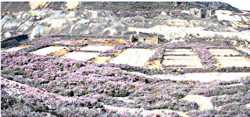
*The pans on Parys Mountain where iron was used to precipitate out copper from a leaching solution.*
