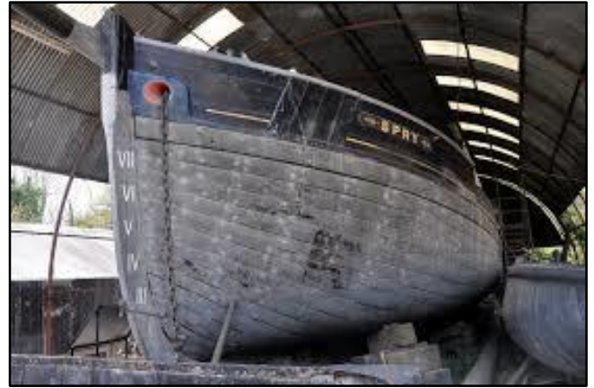
The Spry, recovered as a rotting hull from the Diglis canal basin on the River Severn at Worcester in early 1982. Rebuilt fully to her original river-worthy condition she was successfully sailed, several times, in the Severn estuary, before returning to the Ironbridge Gorge Museum site at Blists Hill.
